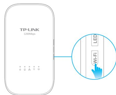
3. When the 2.4GHz Wi-Fi LED and 5GHz Wi-Fi LED on the extender blink quickly for 3 seconds, and then stay on, it's done!
