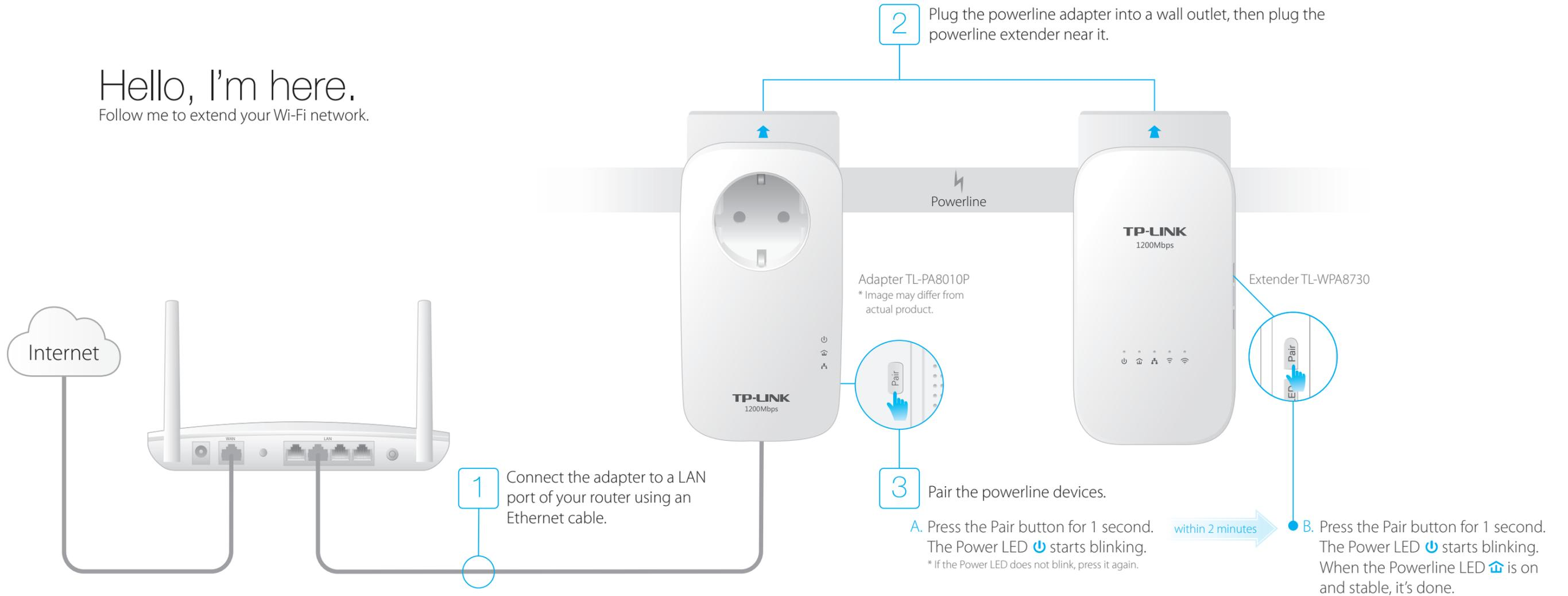
4 Find the Wi-Fi Info Card in the package, then relocate the powerline extender to a wall outlet in the Wi-Fi "dead" zone. Connect to the Wi-Fi using the SSID and password on the card.
